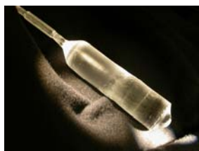
Fig. 2. LSO:Ce boule doped with 0.1 at% Ca. Note the good diameter control.
