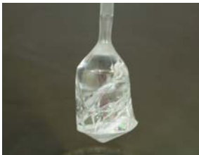
Figure 5 LSO:Ce boule doped with 0.4 at% Ca and 0.2 Zn. This Zn concentration is enough to delay, but not suppress, the onset of acentric growth.
