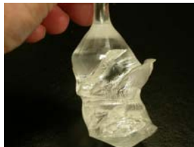
Figure 4 LSO:Ce boule doped with 0.4 at% Ca, exhibiting unstable growth despite a convex interface.
