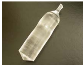
Fig. 3 LSO:Ce boule doped with 0.3 at% Ca, exhibiting stable growth.
