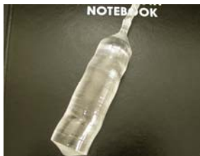
Figure 6 LSO:Ce,Ca,Zn with 0.4 at% Ca, 0.6 at% Zn. Note that growth was significantly more stable.
