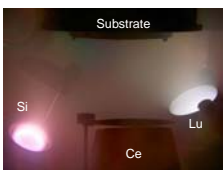
Figure 2. Picture of sputter chamber during processing. Gun targets and substrate holder are labeled.
