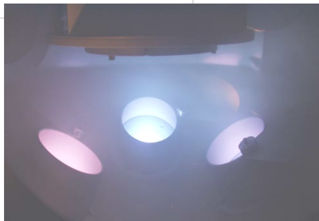
Figure 1. The sputtering system in the process of depositing a Y_3Al_5O_{12}:\text{Gd} library.
